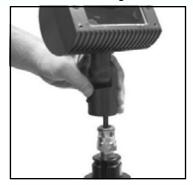
Attach fixture unto coupling. Connect fixture cable to main system cable with a KLV410 Sealed Connector (Part No. 95484).
