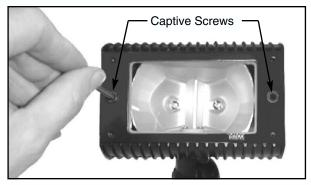
3. To install lamp, loosen the two (2) captive screws on lens frame. Install lamp of type and wattage shown on fixture label and chart on page 2. Replace lens frame assembly making sure gasket fits into the recess properly. Tighten opposing screws progressively & evenly. (Step 3 not required on L.E.D. version, for L.E.D. fixture skip to step 4).
